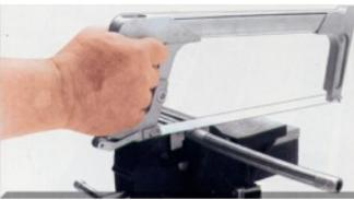
Cut the PTFE hose to the lengths determined in Step 1. Wrap the hose with "Gray" or masking tape at the length desired. Hose may be cut with a hack saw, if you have a 32-teeth-per-inch blade, otherwise a Beverly Shear, radiac, or chop saw will work fine. You want to keep the braids from fraying. After the cut, carefully remove the tape and trim from the frayed ends if necessary.
