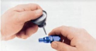
8. Hold the hose and not the socket, start the hose on the nipple of the hose end, with a gentle motion. Continue pushing on the hose until the threads can be engaged. Some sizes may require the use of some force to engage the threads at this point.
