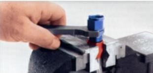
It doesn't matter which portion (the socket or the nipple) is secure in the vise. Using a suitable wrench tighten the socket threads onto the cutter. An adjustable “Crescent” type wrench is not recommended, as it may slip and damage the outside of the hose end.
