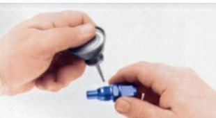
It is very important to lubricate the inside of the hose/socket assembly, and the outside of the cutter threads with any assembly lube, anti-seize compound, or 30 wt. Motor Oil. W/D-40 is not recommended!
