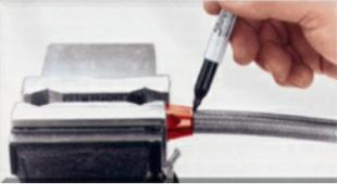
It is important to mark the outside of the hose at the end of the socket. This will show you if the hose has “pushed out” of the socket during assembly, and if so, will leak when used.
